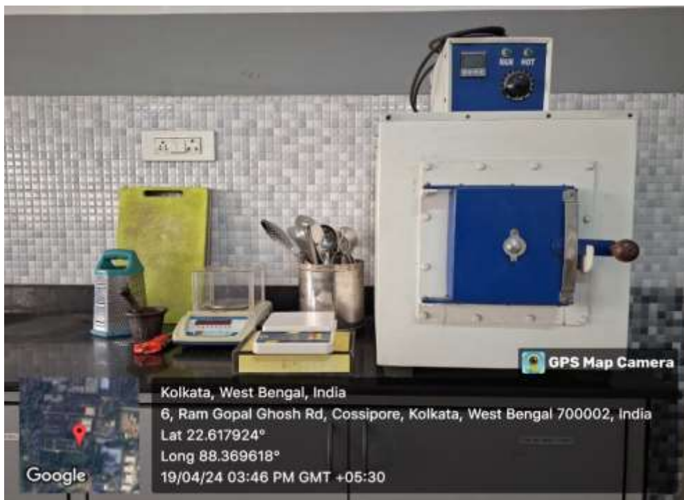
(From left to right: precision balance, electronic compact scale, hot air oven along with some other)
